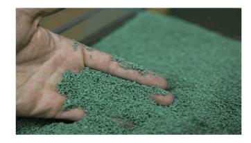
Photo 38: EPDM 'Bionic' infill (Source MILOS)
