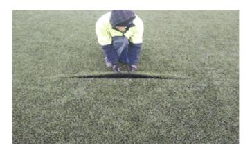
Photo 34: Example of seam failure
