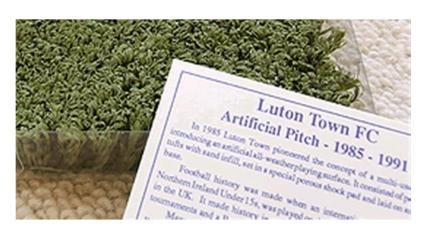
Photo 20: 2<sup>nd</sup> Generation Synthetic Turf (source: Cranfield University <u>www.cranfield.ac.uk</u>)
