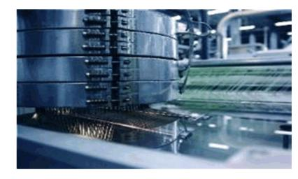
Photo 32: Extrusion Process producing mono-filament yarn
