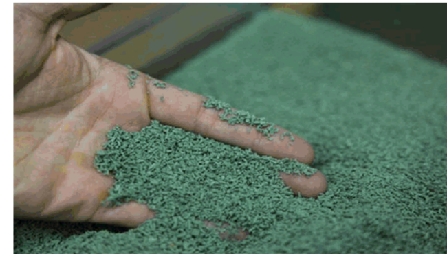
Photo 38: EPDM 'Bionic' infill (Source MILOS)
