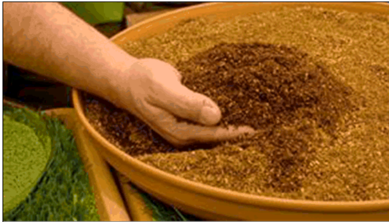
Photo 39: Organic Infill (Source: Limonta)
