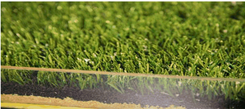
Photo 35: Example of a mixed profile of sand and rubber infill
