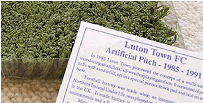
Photo 20: 2 nd Generation Synthetic Turf (source: Cranfield University www.cranfield.ac.uk )
