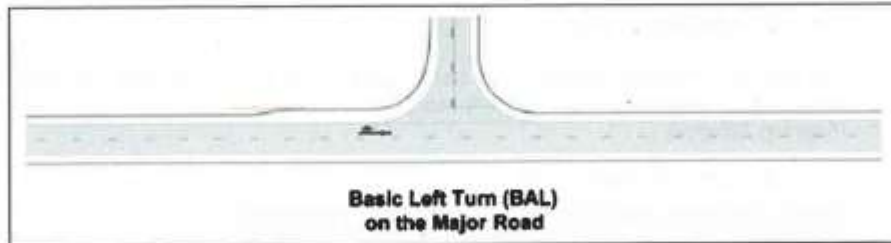
Figure 10: Rural basic left turn treatment
