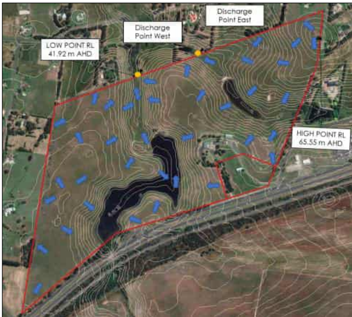
Figure 9: DRAINAGE STRATEGY (Not to scale)
