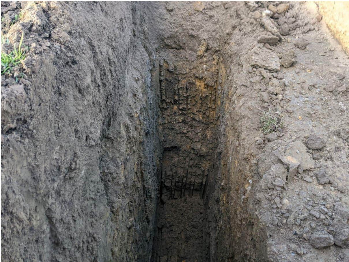
Photograph 21: View of TP06. Trace fill inclusions were observed within test pits within the filled area.
