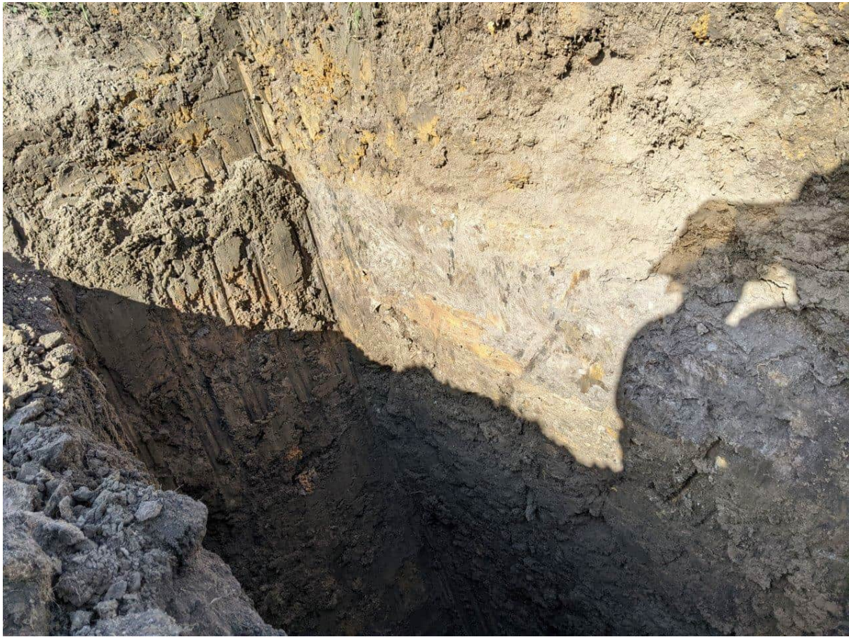
Photograph 19: View of TP04. Trace fill inclusions were observed within test pits within the filled area.
