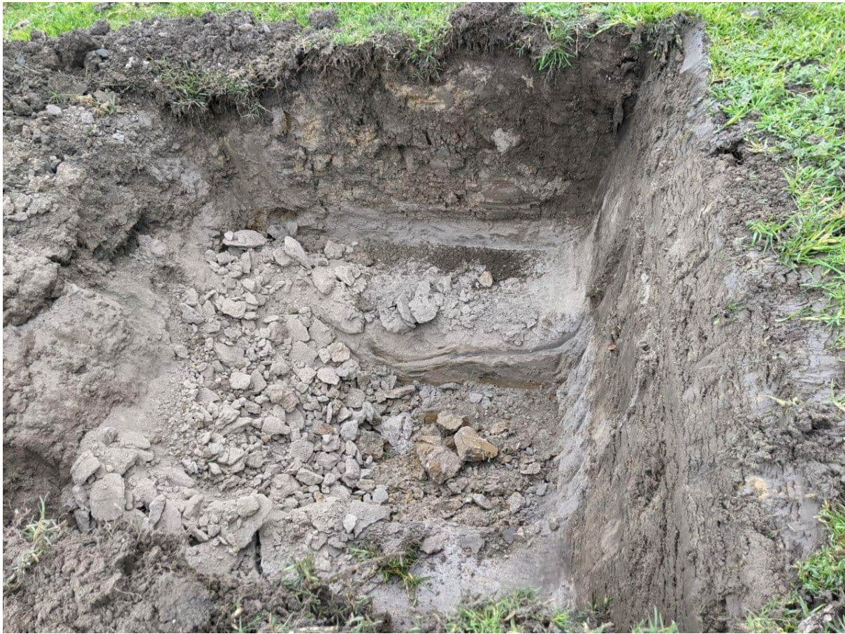
Photograph 17: View of TP02. Trace fill inclusions were observed within test pits within the filled area.
