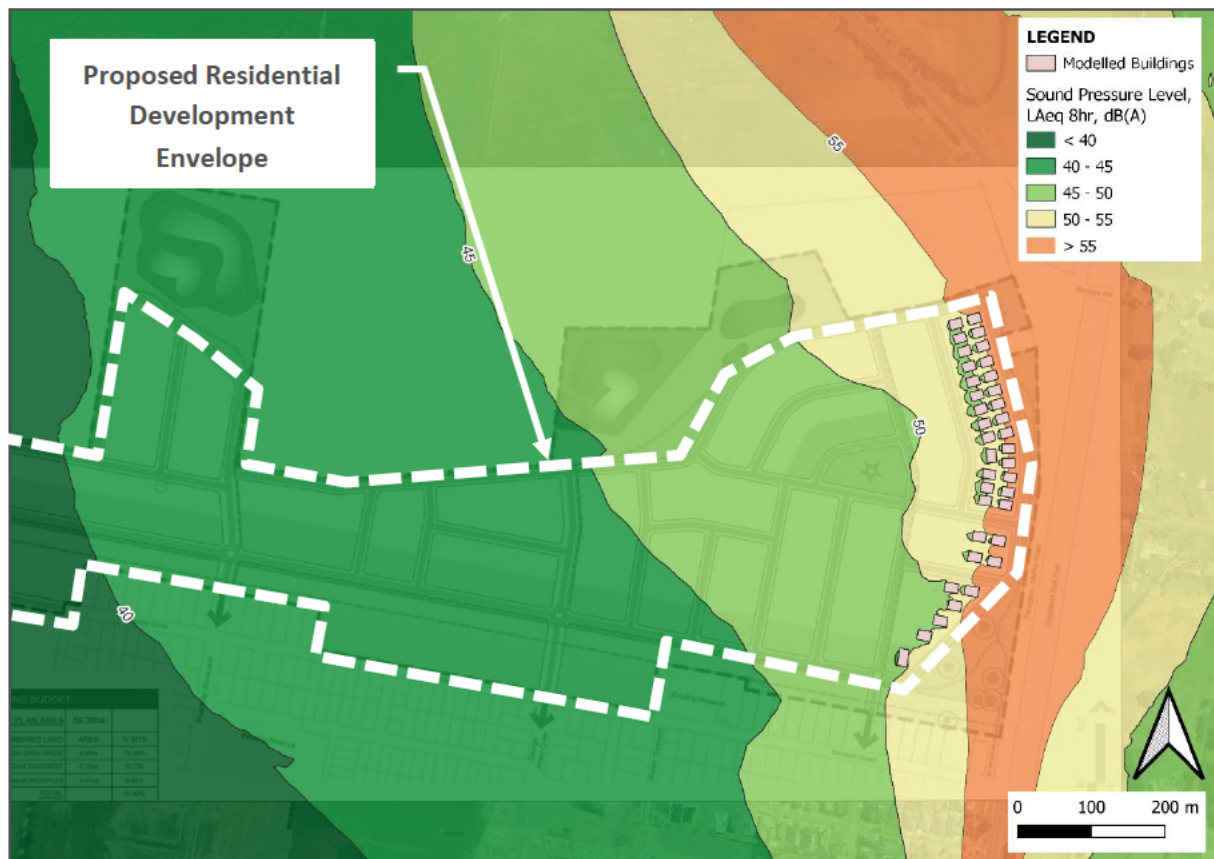
Figure 5 Calculated Year 2037 L_{Aeq,8hr} Traffic Noise Contours
