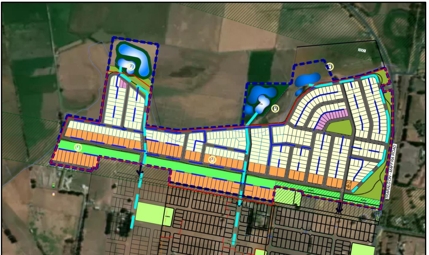
Figure 4: Drainage Arrangement Option
