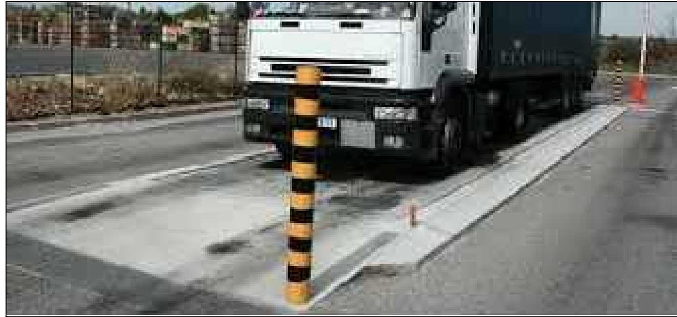
TYPICAL WEIGH BRIDGE 100 TONNE CAPACITY
