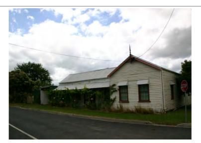
**DESCRIPTION** The former Selector's Arms Hotel is a weatherboard building, which is T-shaped in plan. It comprises a long elevation facing Austin Street with a double transverse gable roof and a street verandah. At the western end is a single traverse gable with a finial in the gable end. Windows are multiple pane double hung sash and there are four, four panelled doors opening onto the verandah. The building is built to the street boundary.
