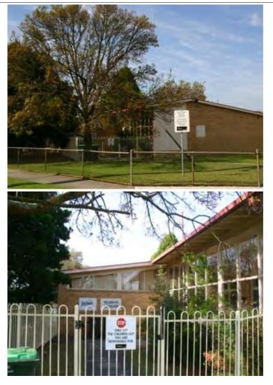
**DESCRIPTION** This is a post war brick kindergarten. It has a shallow pitch gabled roof and timber framed windows. It appears to be externally intact apart from the enclosure of the porch/verandah. This has been done sympathetically with the addition of timber framed windows along the north elevation. The play area on the east side of the building was not inspected and so it is not known whether the original playhouse has survived or how original the layout of the playground is.
