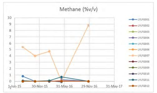
Figure 11 Methane concentrations in perimeter bores.
