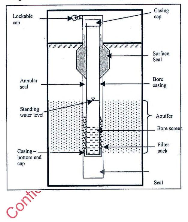
Figure 1: Groundwater monitoring bore
