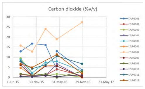
Figure 12 Carbon dioxide concentrations in perimeter bores
